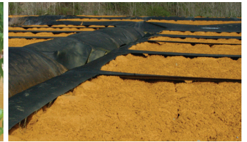
Iron oxide settles in the ponds and is harvested and sold for commercial use.
